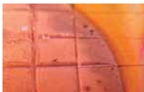
Cut edge is smooth and peel-off was not observed.
